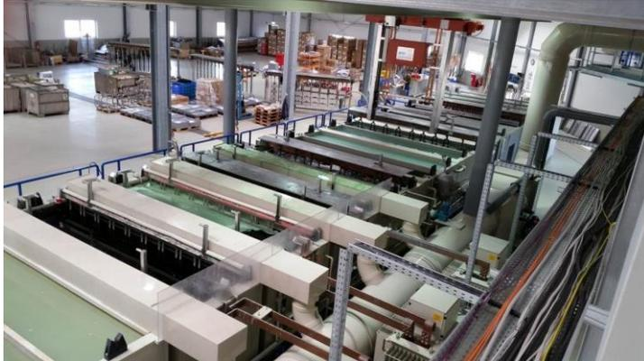
**Figure 9 - Rinsing baths in the galvanic industry**
